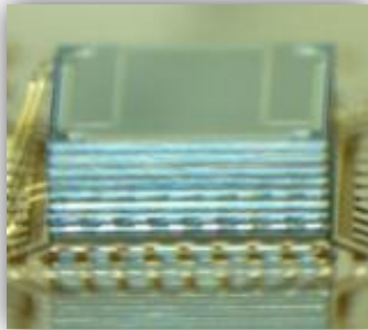
Fig.8: a 33 \mu F Capacitor in a package size of 4.8mm*4.4mm*2 mm
